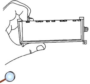
11. On bottom side of plastic bracket assembly, directly below the 2 large, plastic snap features, locate the under cut edge. Pull this under cut edge outward, up and over the side of the module.
